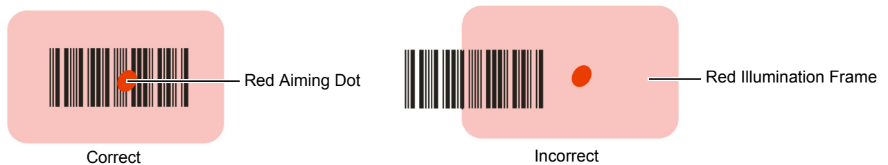
Figure 1-10 Imager Illumination Frame
