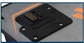
Floating Docking Connector protects against damage.
