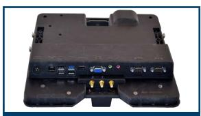
Rear-facing port replication protects cable connections while integrated strain relief protects from accidental disconnects
